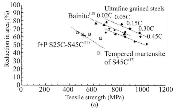
**Relationship between reduction in area (RA) and tensile Strength of ferrite + pearlite steel (■)<sup>(9)</sup>, bainite steel(Δ)<sup>(10)</sup> tempered martensite (●)<sup>(9)</sup>, and ultra-fine-grained steel (◆).**
