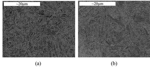
Fig.5. SEM microstructure of BC 4149 (a) 500°C and (b) 600°C .
