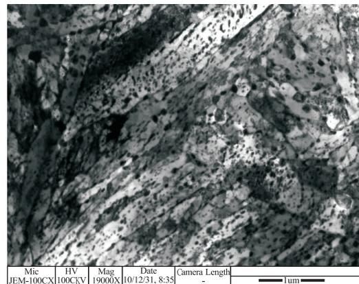
Fig.6. TEM microstructure of BC 4149, tempered at 600°C.
