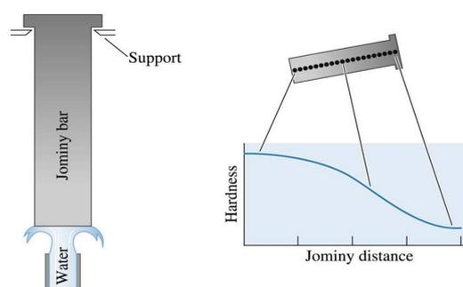
**Fig. 2.** The Jominy end-quench test.
